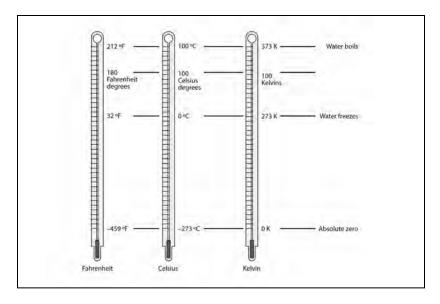
water are factors in establishing the scale's range. There are 100 degrees between the temperate at which water freezes (273.16 K) and boils (373.16 K). Each unit on this scale, called a Kelvin rather than a degree, is equal to a degree on the Celsius scale. For this reason, just the K, not the degree symbol (°), is used when reporting temperatures in Kelvin. There are no negative numbers on the Kelvin scale, as the lowest number is 0 K.
